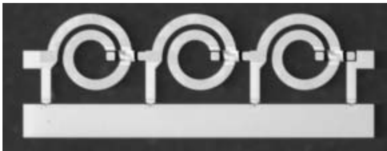
Figure 4.2: An X-band quasi-distributed analog phase shifter.
