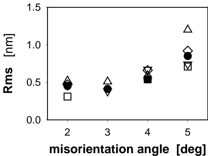
Rms of 2  $\mu\text{m} \times 2 \mu\text{m}$  AFM images:
